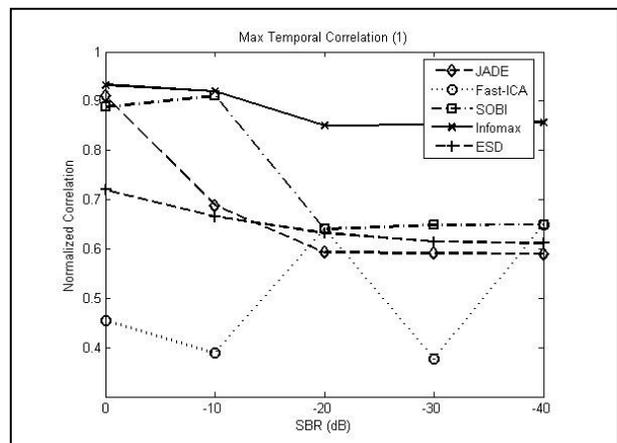
Figure 6: Temporal normalized correlations for the cat data with synthetic stimulus, correlated against reference signal 1. Infomax clearly outperforms the rest of the ICA algorithms.
