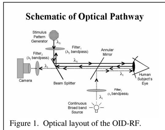
Figure 1. Optical layout of the OID-RF.
