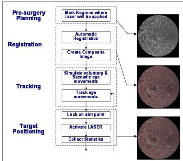
Figure 1. Block diagram of the computer-based simulation.
